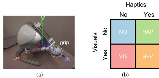
Figure 1: (a) A photo of the Novint Falcon used in our experiments. The device can track user movement of the grip and apply forces in 3D. (b) The abbreviations for each of the four between-participant conditions. NO - No haptics and no visuals (blue), HAP - haptics and no visuals (green), VIS - no haptics with visuals (pink), and H+V - haptics and visuals (orange).
