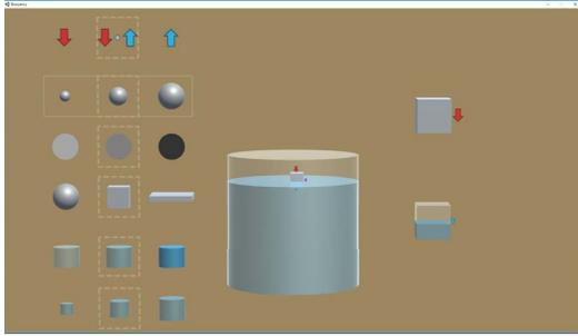
Figure 2: A screenshot of the simulation used in our experiment. The property selection menu is shown on the left side of the screen. In the center is the container, liquid, and buoyancy object. In this image, the object is set to a cube and is floating near the center of the container. On the right side of the screen is a visualization of the buoyancy object (top) and the volume of the displaced liquid (bottom).
