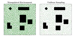
Figure 2: *Left:* An environment with obstacles (black) and the constrained Delaunay triangulation (green) of the free space. *Right:* The vertices (green) of the constrained Delaunay triangulation that lie inside the free space. These vertices are the sampled points at which we compute visibility polygons to describe the structure of the environment and compute our ENI metric.
